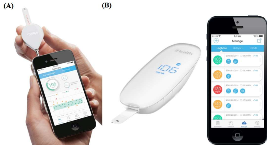
Smartphone-based blood glucose meters developed by iHealth Inc.
